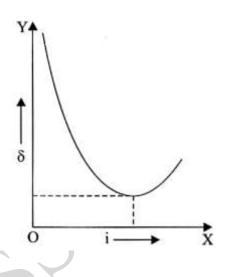
When the prism is placed in the minimum deviation position, the refracted light is parallel to the base of the prism. At this position, the incident and the emergent rays are symmetrically inclined. To sum up, when the prism is placed in the minimum deviation position, the ray of light passes symmetrically through the prism.
