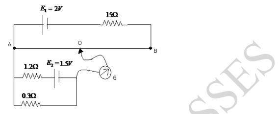
**SOL:** <u>Principle of potentiometer:</u> The potential difference across any two points of current carrying wire, having uniform cross-sectional area and material, of the potentiometer is directly proportional to the length between the two points, i.e.,  $V \propto l$
