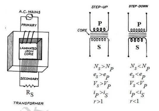
The **ac device** used to **transform** an alternating voltage from one value(High voltage) to another value (Low voltage) and vice-versa is called **transformer**.
