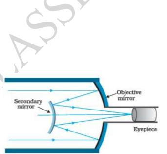
of equivalent optical quality, and can be supported over its entire back surface, not just over its rim. One obvious problem with a reflecting telescope is that the objective mirror focusses light inside the telescope tube. One must have an eyepiece and the observer right there, obstructing some light (depending on the size of the observer cage).
