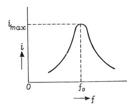
23) An alternating voltage of frequency f is applied across a series L-C-R circuit. Let  $f_r$  be the resonance frequency for the circuit. Will be current in the circuit lag, lead or remain in phase with the applied voltage when (i)  $f > f_r$  (ii)  $f < f_r$ ? Explain your answer in each case.
