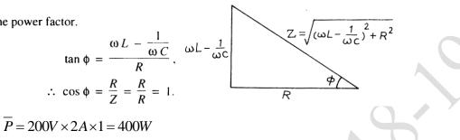
16) A resistor of 12  $\Omega$ , a capacitor of reactance 14 $\Omega$  and a pure inductor of inductance 0.1 H are joined in series and placed across 200 V, 50 Hz ac supply. Calculate (i) the current in the circuit (ii) phase angle between current and voltage. Take  $\pi = 3.$  [CBSE 1993]
